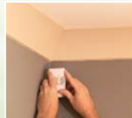
Wireless Motion Sensor Mounted near the point of use and operates the recirculation system with the detection of motion and designed to detect full-body movement up to 30 feet (turns recirculation on/off in five minutes)
