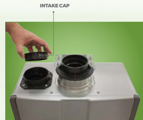
For PVC/CPVC configurations, the intake cap is removed and discarded. With this option, installers can use 3- or 4-inch PVC/CPVC pipe for the intake and exhaust.
