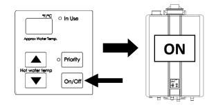
**1** Press push button. Module LED blinks **GREEN** and pump turns on.
