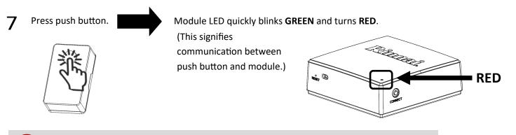
IMPORTANT: After pressing push button, DO NOT press it again until 5-minute timer is complete (as explained in next step).
