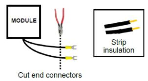
b Connect module wires to water heater controller cable (included in water heater packaging) using wire nuts or other approved wire connectors. Wire Nuts Controller Cable
