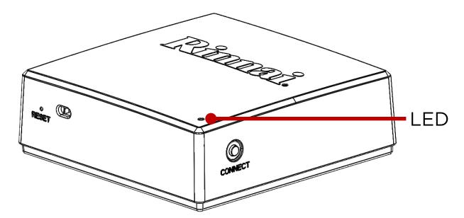
Press and hold down the **Connect** button on the module until the LED turns GREEN.
