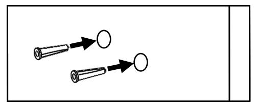
Insert the screws (supplied) into the anchors and fasten to the wall leaving 1/4 in. exposed.
